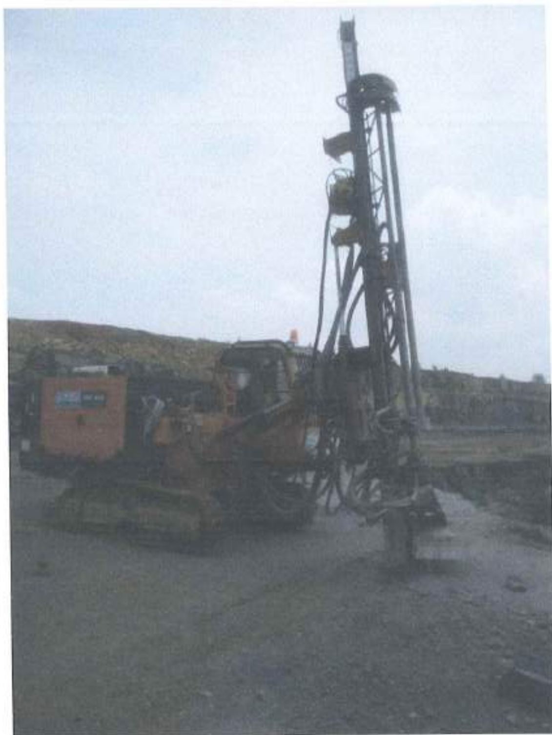
DTH - wet drilling at Karunda Limestone mine
