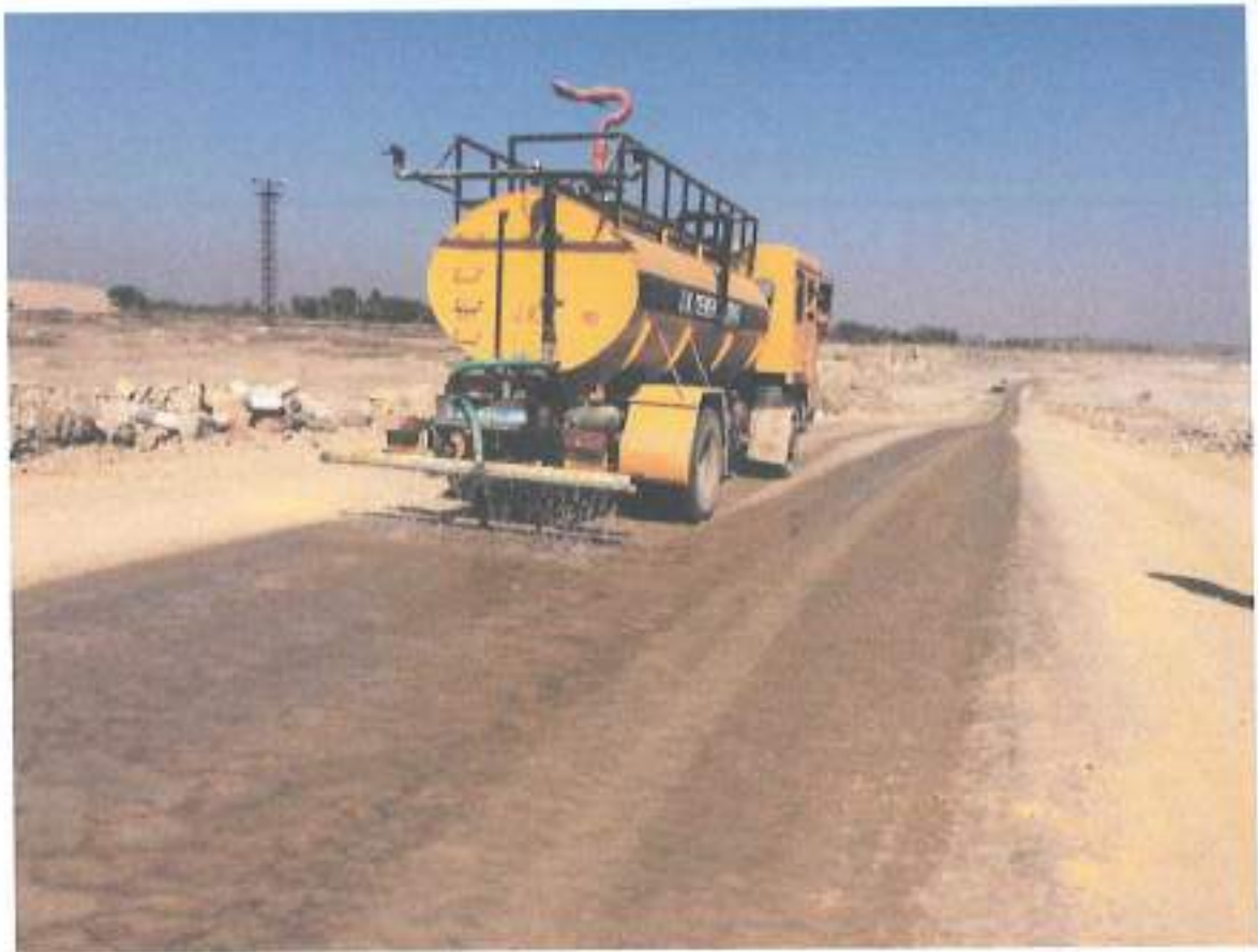
Water sprinkling through water tanker at Karunda limestone mine
