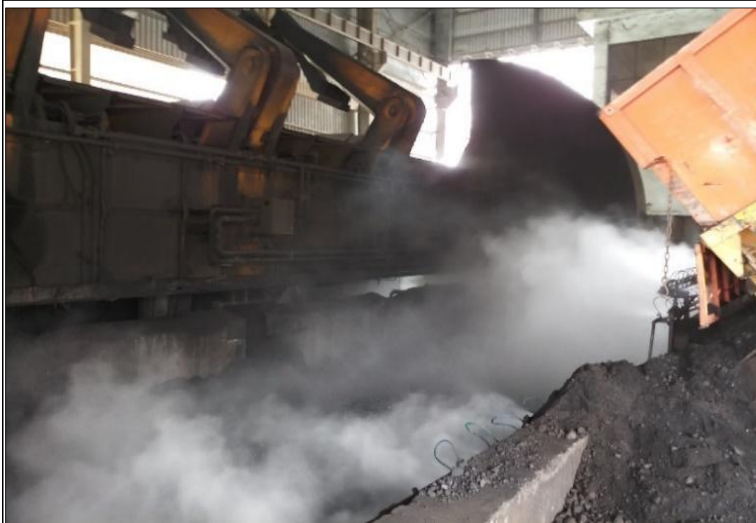
Water spraying system (fog system) at coal unloading point
