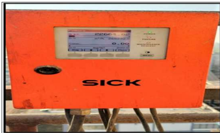
Picture 9- Continuous Emission Monitoring Systems (CEMS) installed and Data uploading in CPCB & MPPCB server
