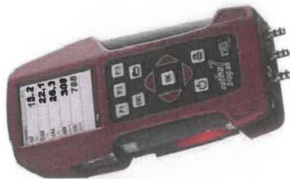
FIGURE-1 PORTABLE COMBUSTION GAS ANALYSER
