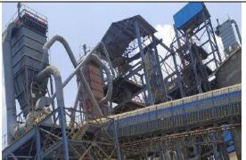
Covered transportation and conveying system for raw material and closed bulkers for carrying fly ash is being practiced to prevent spillage and dust generation. Photographs of Fly Ash Unloading System is enclosed below.
