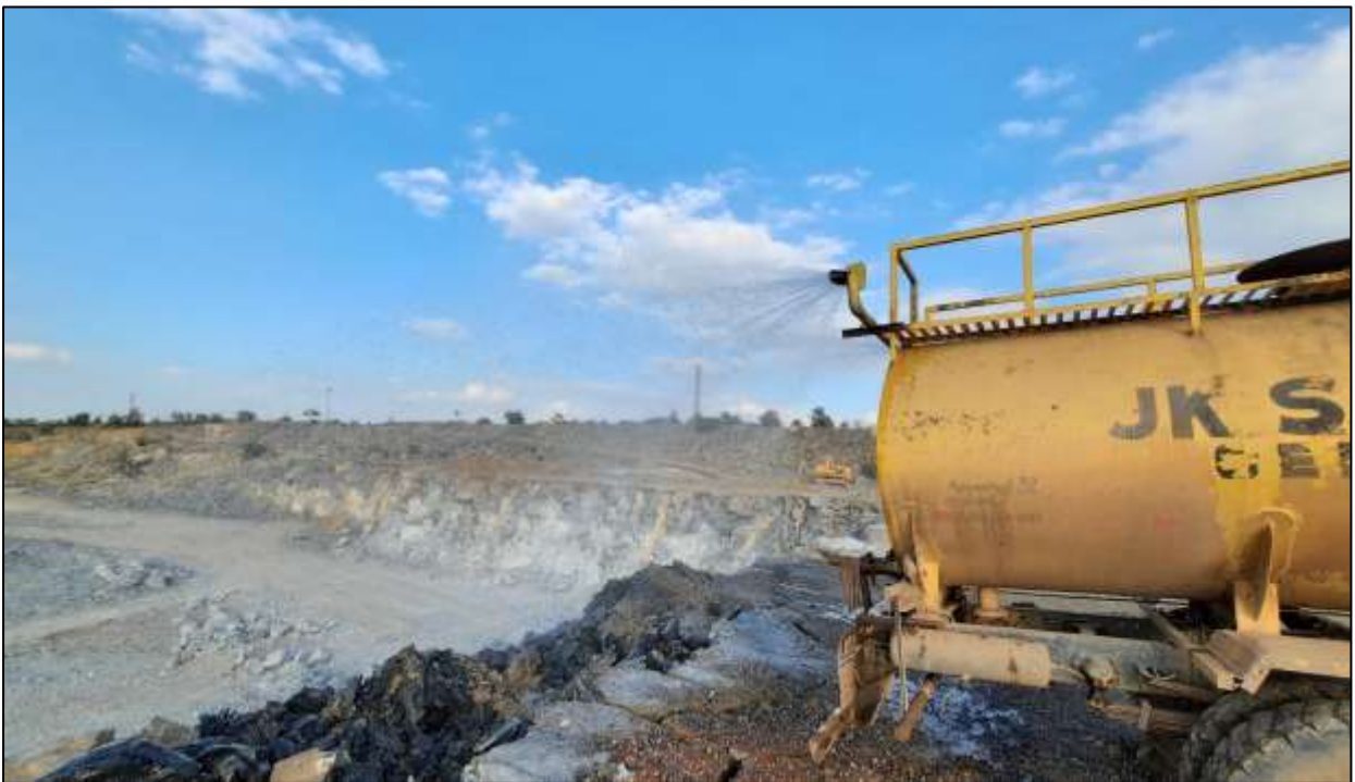
Water sprinkling on blasted muck pile to reduce dust generation
